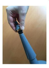
Hold the nozzle cap tight and use the slotted screwdriver to turn the valve stem off the nozzle cap.
