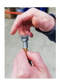
Hold the star bit tight and use the slotted screwdriver to turn the valve tube off the star bit.
