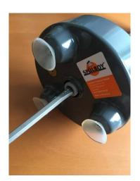
Insert a slotted screwdriver into the opening.
